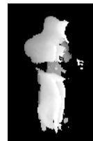
Figure 1: Output frame from history algorithm. As the grayscale gradient suggests, object is moving to the right.
