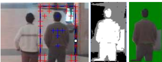
Figure 4: Calculation of the histogram mask . Leftmost image shows placement of template markers on target object. Notice the placement of foreground (blue) and background (red) markers. Middle image shows resulting mask after region growing was applied on foreground and background markers (foreground label is white, background is black and neutral label is gray). Rightmost image shows an overlay of the mask on the original image, where foreground pixels kept their original color and background and neutral pixels are green.
