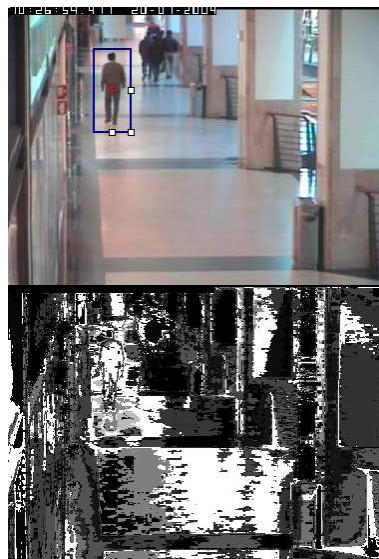
Figure 2: External box histogram : calculation of initial box histogram (box depicted as a blue rectangle on the top image) and corresponding back projection (bottom image) on the same frame. Shows low accuracy of histogram, as background pixels are contained within the bounding rectangle.
