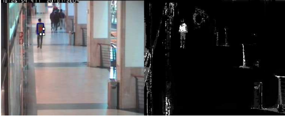
Figure 3: Internal box histogram : calculating the initial histogram based on a region within the object being tracked rather than bounding the entire object yields better back-projects (right image).
